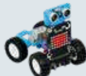
Vertical Steering Robot with Ultrasonic Sensor
